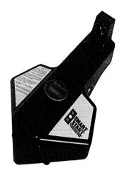
The SMART START IN-HOM unit is an affordable alternative for the offender who needs alcohol monitoring. The IN-HOM monitor is an alcohol specific fuel cell based device equipped with a camera allowing for photo identification of the person submitting the test.
